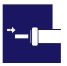
**Insert the hose** past the clamp and internal O-Ring gasket up to the tube stop.
